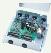
Serial parallel device controlling outdoor units, up to 4 units.
