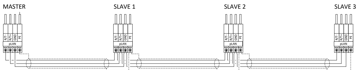
Figure 6.3. Building a pLAN network.
